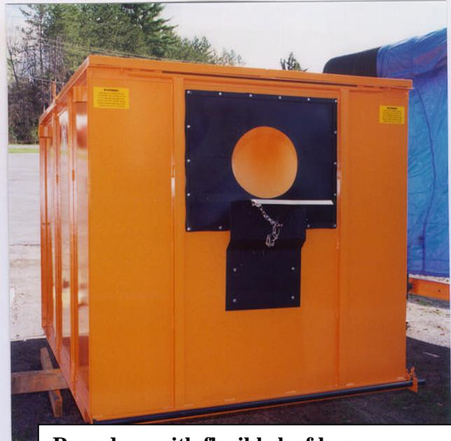
**Rear door with flexible leaf box connector and discharge hose/tube support. Sides and rear door are constructed out of 10-gauge steel.**
