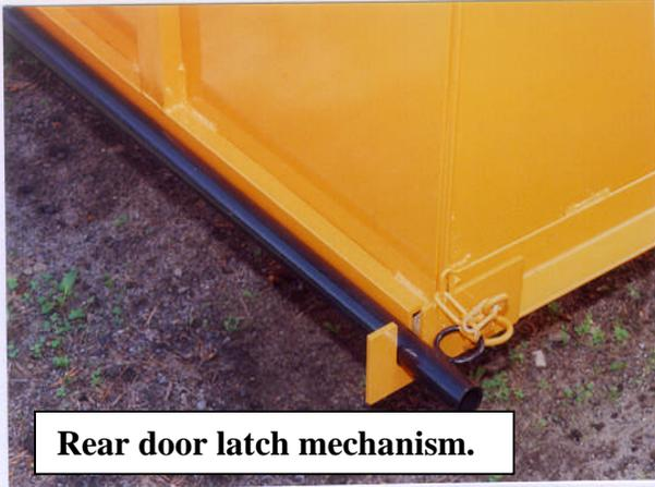
**Rear door latch mechanism.**
